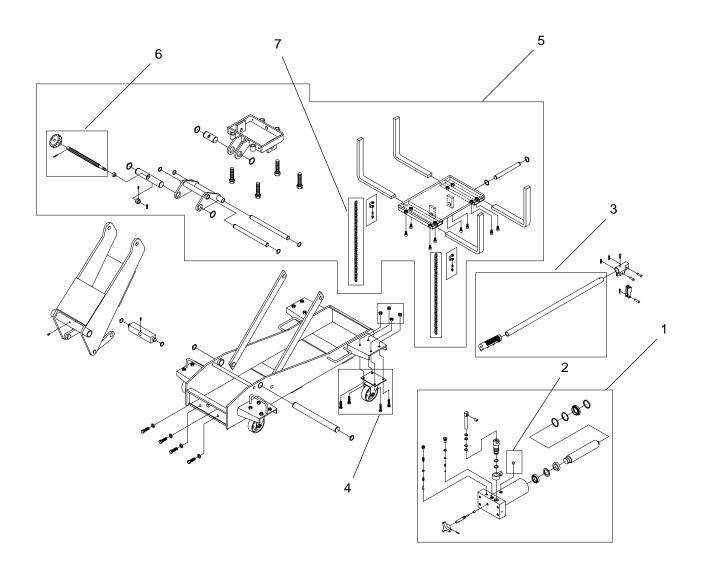
Figure 4 - Replacement Parts for Model 43000
